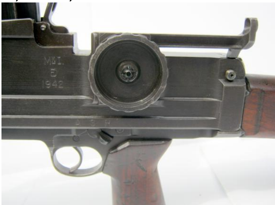
Marks "Mk I Enfield 1942", rear sight, change lever "A,S,R"
